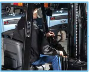
The small-diameter steering wheel with the full hydraulic power steering system provides excellent maneuverability.
