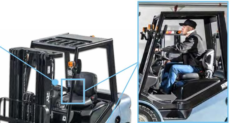
The large assist grip, low step make getting on and off more smooth. This can help reduce the operator's fatigue.
